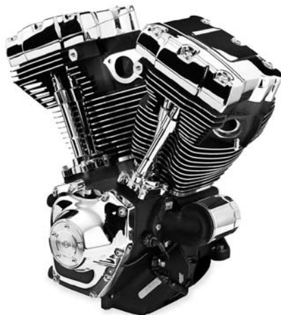
D. Black and Chrome 1450cc Twin Cam 88 Engine
